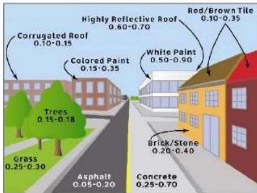
Fig.5 – Illustration of urban surfaces with different albedo levels
