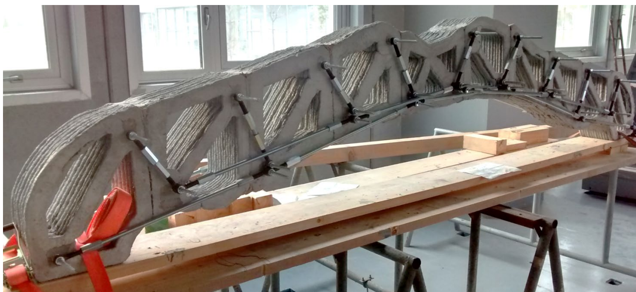
Fig. 6 - 3D printed reinforced concrete curved beam (University of Naples)
