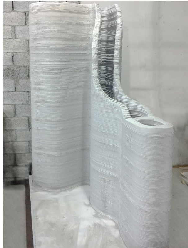
Fig.1 - 3D printed element realized with Cobod International
